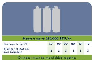
or allow simultaneous vapor withdrawl from all cylinders
